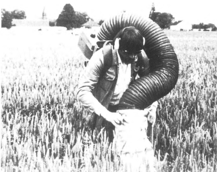
Fig 5 A D-Vac suction net being used to collect arthropods from the leaves of wheat
