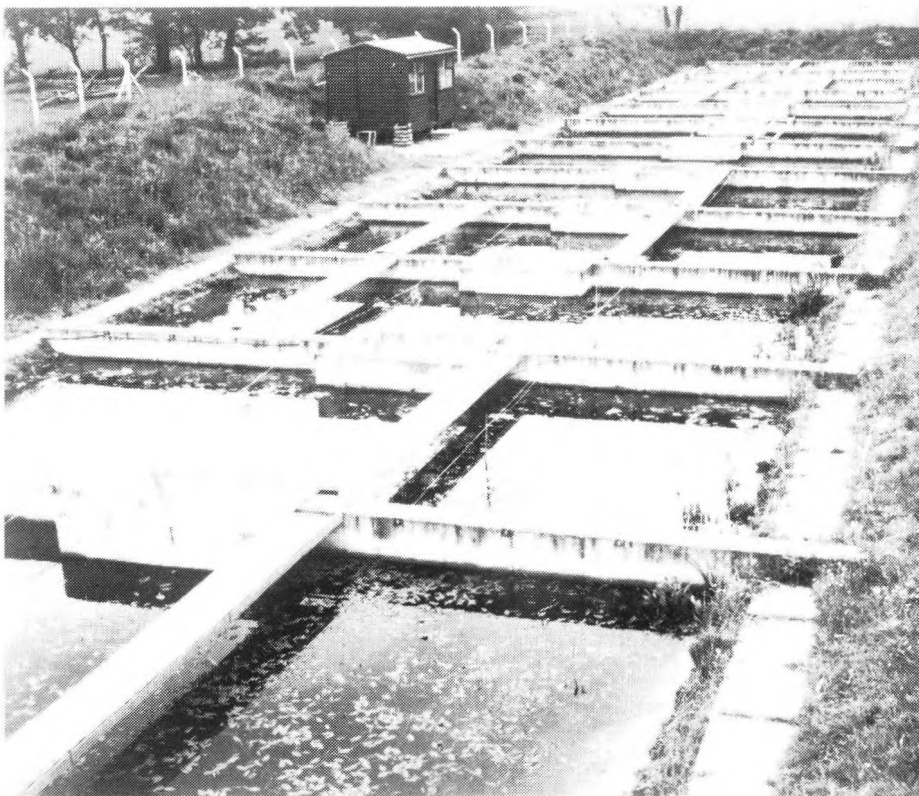
Fig 4 Outdoor ponds used to evaluate fate and effects of pesticides in aquatic environments
