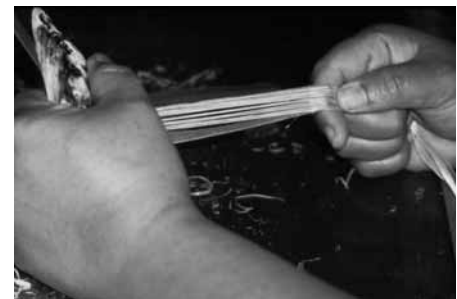
Fig. 2 Traditional haro method of stripping fibre (muka) from harakeke leaves, using the sharp edge of a shell. Photo: Sue Scheele.
