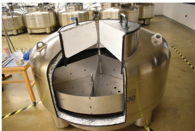
Fig. 5 Dissected 1500 litre liquid nitrogen dewar showing the turntable on which sample racks are housed and thick insulation to maintain temperatures at -196^{\circ}\text{C} .
